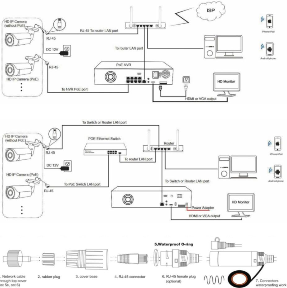
Figure 2: Working With PoE switch and NVR
